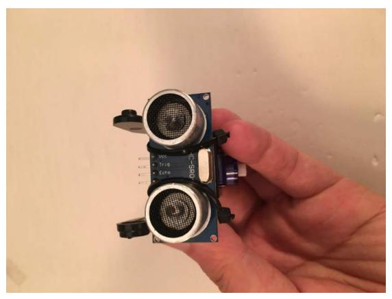
In order to fit the holder, we need cut the rubber holder cross as the same length on four direction.
