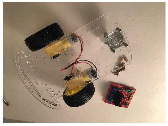
Before you fix the screw, passing the wire on the motor through the board helps your next step.
