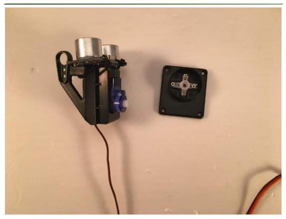
**Note:** when you fix servo holder on it's base(black plastic of the right on above the picture), you need read the actual code to adjust your servo on the most correct angle.
